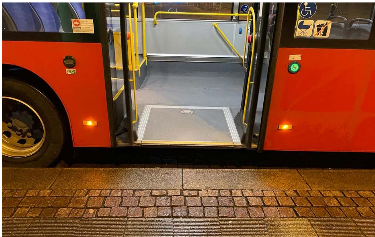
Image 6.17 Accessible buses with folding ramp Photo Credits: Dr. Gaurav Raheja
