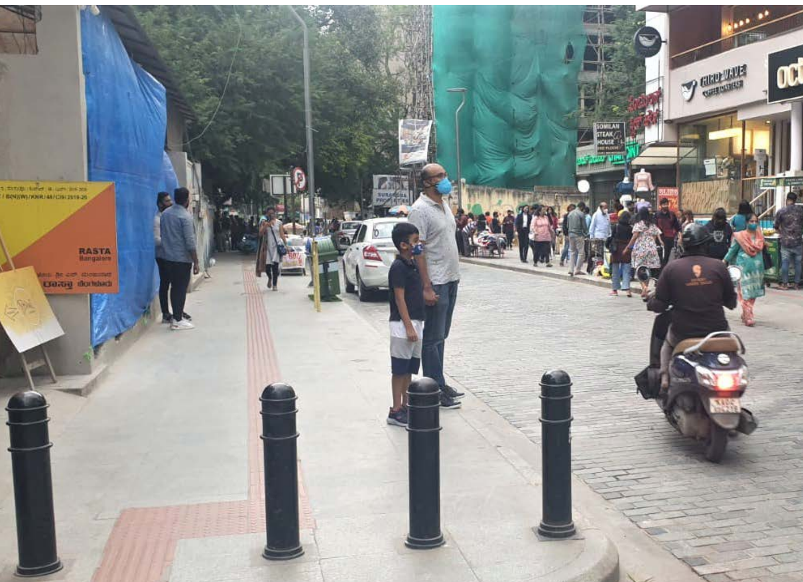
Image 3.28 Typical bollard placement for accessible sidewalk with tactile pavers: Church Street Photo Credits: Shreya Shetty
