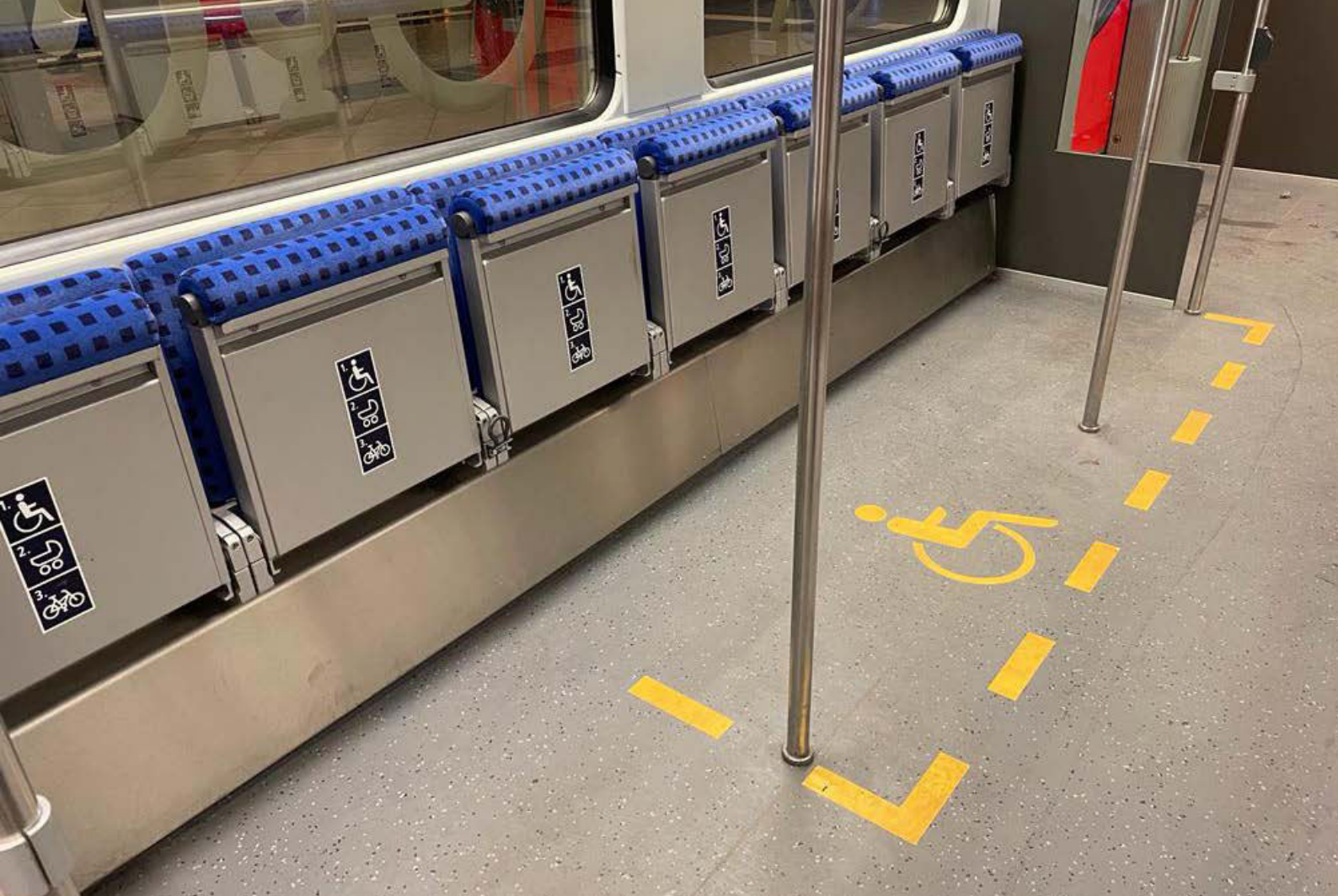
Image 6.22 Accessible metro rail coach design and seating Photo Credits: Dr. Gaurav Raheja
