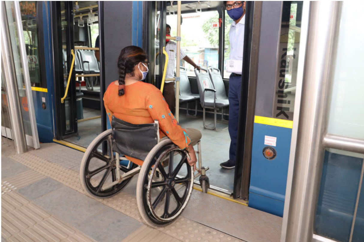
Image 6.16 Accessible buses with level approach: Ahmedabad BRTS Photo Credits: CPWD
