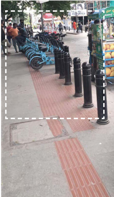
Image 2.21 Obstructions on tactile pathway
