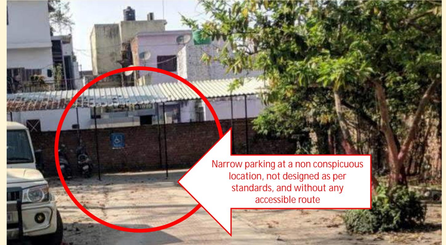
Narrow parking at a non conspicuous location, not designed as per standards, and without any accessible route
