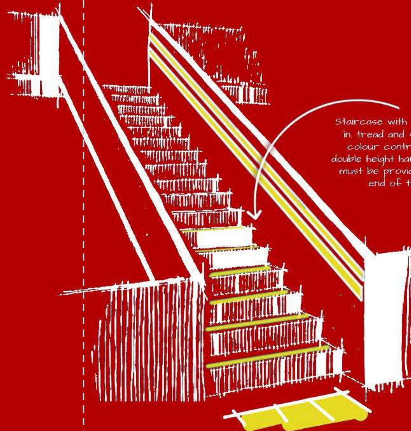
Staircase with regular steps of 9 in. tread and 4.5 in risers, with colour contrasting strips and double height handrails. Warning tiles must be provided at beginning and end of the staircase
