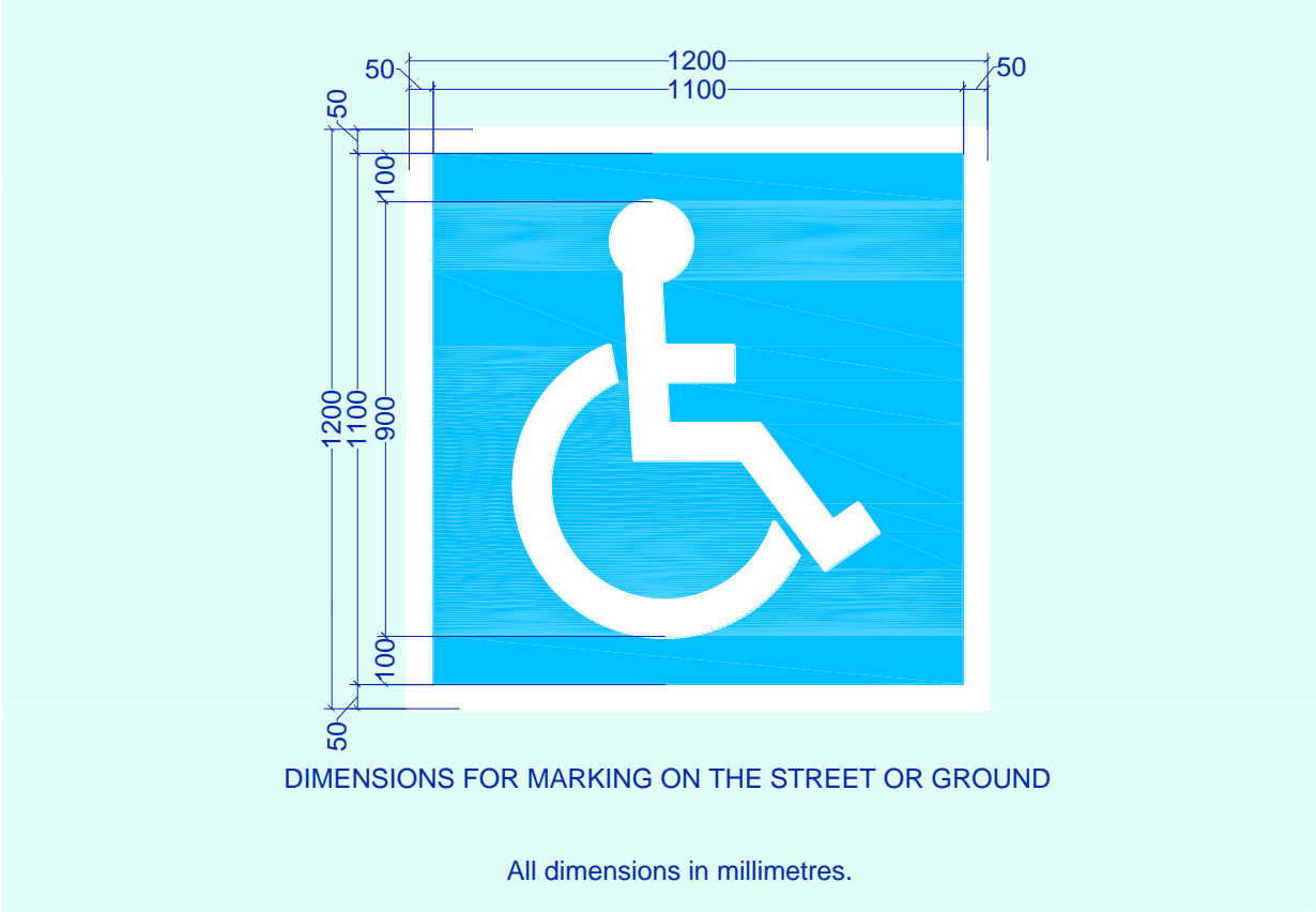
Figure 10: Details of on-floor International Symbol of Accessibility
